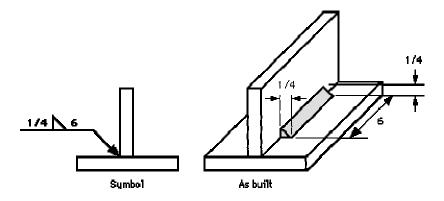
If no length is given, then the weld is to be placed between specified dimension lines (if given) or between those points where an abrupt change in the weld direction would occur (like at the end of the plates in the example above).
