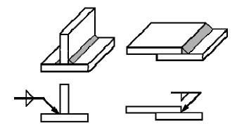
The perpendicular leg of the triangle is always drawn on the left side of the symbol, regardless of the orientation of the weld itself. The leg size is written to the left of the weld symbol. If the two legs of the weld are to be the same size, only one dimension is given; if the weld is to have unequal legs (much less common than the equal-legged weld), both dimensions are given and there is an indication on the drawing as to which leg is longer.
