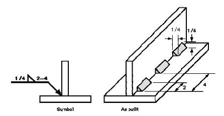
Notice that the spacing, or **pitch**, is not the clear space between the welds, but the center-to-center (or end-to-end) distance.
