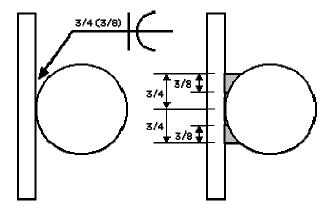
Common supplementary symbols used with groove welds are the **melt-thru** and **backing bar** symbols. Both symbols indicate that complete joint penetration is to be made with a single-sided groove weld. In the case of melt-thru, the root is to be reinforced with weld metal on the back side of the joint. The height of the reinforcement, if critical, is indicated to the left of the melt-thru symbol, which is placed across the reference line from the basic weld symbol.
