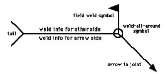
The horizontal line--called the reference line--is the anchor to which all the other welding symbols are tied. The instructions for making the weld are strung along the reference line. An arrow connects the reference line to the joint that is to be welded. In the example above, the arrow is shown growing out of the right end of the reference line and heading down and to the right, but many other combinations are allowed.
