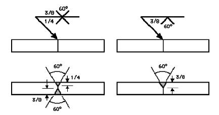
If the penetration of the weld is to be greater than the depth of the groove, the depth of the **effective throat** is given in parentheses after the depth of the V.
