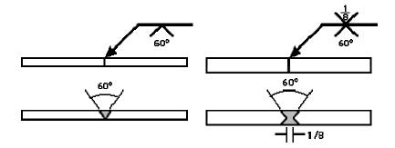
If the depth of the V is not the full thickness--or half the thickness in the case of a double V--the depth is given to the left of the weld symbol.
