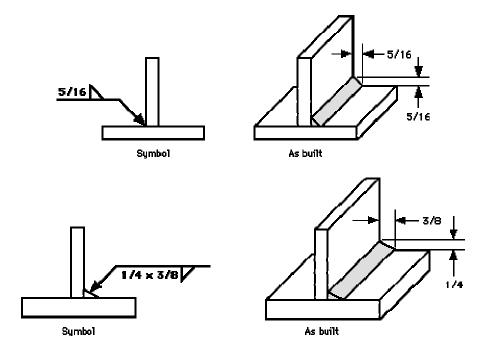
The length of the weld is given to the right of the symbol.
