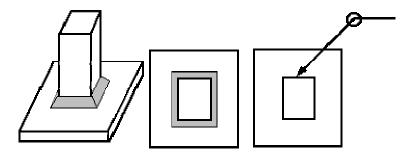
The tail of the weld symbol is the place for supplementary information on the weld. It may contain a reference to the welding process, the electrode, a detail drawing, any information that aids in the making of the weld that does not have its own special place on the symbol.
