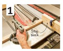
■ Use a table saw and miter gauge to cut parts to length. Clamp a stop block to the fence so the parts will be exactly the same length. It's important that the stop block be far enough behind the blade to prevent binding and kickback.
