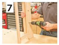
● Once you have sanded the parts, bore pilot holes for the screws in the frame and shelf. Then attach the shelf to the frame with glue and four No. 6 x 1-1/2-in. screws driven through the back of the frame (see illustration).
