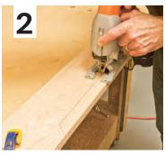
Lay out the cutout section on the bottom rail with a combination square and a pencil. Clamp the workpiece to your workbench; then use a jigsaw and a fine-tooth blade to make the cut.
