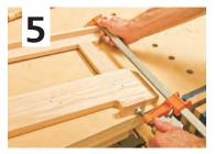
Test fit the frame parts before joining them together. Also, confirm that the dowel holes are deep enough to accommodate the dowels with a little extra space. To prevent marring, use scrap blocks between the clamp jaws and workpieces.
