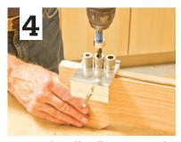
■ Use a doweling jig to center the holes in the rails and stiles. A brad-point drill bit will bore the most precise holes. Not all jigs operate the same way, so be sure to follow the instructions that come with the tool.
