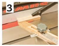
■ Cut the rabbets in the backs of the rails and stiles with a table saw and a featherboard. Set the blade 1/4 in. high and the fence 1/4 in. from the outside edge of the blade. (Note: The blade guard has been removed for photo clarity.)
