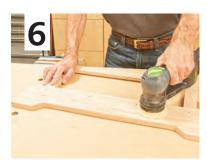
■ Sand the assembled frame thoroughly before attaching the shelf. Progressively use 80-, 120- and 180-grit sandpaper. A randomorbit sander with dust collection is more efficient and less messy than sanding by hand.
