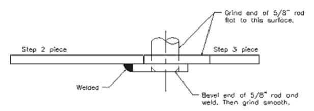
After this is done, see that the two pieces mate up and the holes align with each other. If not, you can grind some material out of the two welded pieces. Don't grind the single piece to less than 3/16 inch (.4762 cm). Place one of the 5.8 inch (1.587 cm) round pieces into the holes and rotate the hinge to make sure it works. Make any adjustments at this time.
