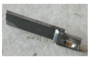
2 Overlap the 1.25 x 1.25 inch (3.175 x 3.175 cm) piece with the hole in it onto the 3 inch (7.62 cm) piece of 3/16 inch (0.4762 cm) flat stock by 0.250 inches (0.635 cm) and weld together. Make sure you weld only the side where the small piece overlaps the longer one.
