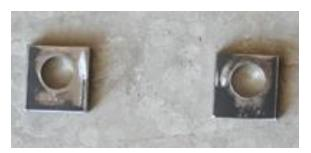
In both of the 1.25 x 1.25 inch (3.175 x 3.175 cm) pieces of 3/16 inch (0.4762 cm) flat stock, drill a 5/8 diameter hole .500 from one end in the center of the piece.
