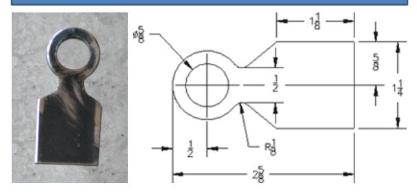
3 Drill a hole in the 2.625 inch (6.667 cm) pieces of 3/16 inch (.4762 cm) flat stock .500 inch from one end in the center of the piece. Grind the end around the hole so there is 3/16 inch (.4762 cm) of material all the way around leaving about 1/2 inch (1.27 cm) in the center of the piece.
