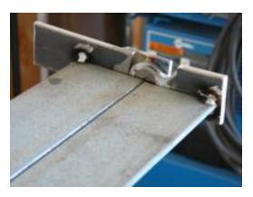
Clamp the two pieces of 25 inch (63.5 cm) x 2 x 2 x 3/16 inch (5.08 x 5.08 x .4762 cm) angle together, center where they come together with the center of the 5/8 inch (1.587 cm) rod and weld to each hinge. The top of the two pieces should be centered top to bottom on the two hinges.
