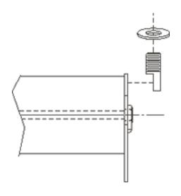
7 Cut the head from the 2 x 3/4 inch (5.08 x 1.905 cm) bolts, grind half way through the bolt about half way up the bolt and weld to the bending side of the hinge. (The piece that does not have the 5/8 inch (1.587 cm) rod welded to it.)
