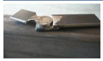
Bevel one end of the 5.8 inch (14.73 cm) rod, line up both pieces and push it through. You should be able to rotate the two assemblies. The beveled end will be on the 1.25 x 1.25 inch (3.175 x 3.175 cm) piece, push it flush and weld, filling in where the bevel is. Grind the other side of the hinge.
