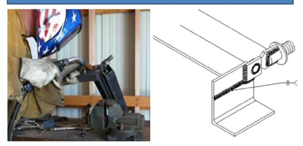
Weld the two 3.5 inch (8.89 cm) long pieces of 2 x 2 x 3/16 inch (5.08 x 5.08 x .4762 cm) angle to the bottom of the other side of the hinge on both sides. This will be the base to clamp the brake to a table.
