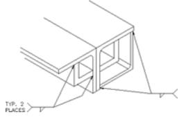
9 Weld the bracing underneath the platens, the 1 x .25 inch (2.54 x .635 cm) angle will be on both sides and the 1.75 x 1/8 inch (4.445 x .3175 cm) angle is only underneath the bending platen, on top of the 1 x .25 inch (2.54 x .635 cm). Use as many clamps as you can while welding these in place.
