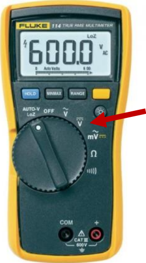
DC Voltage Setting
