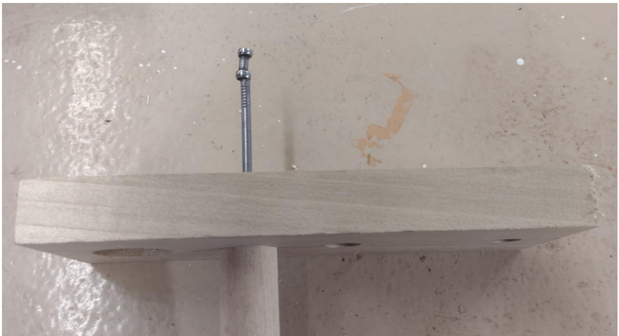
Dowel inserted into the hole.
