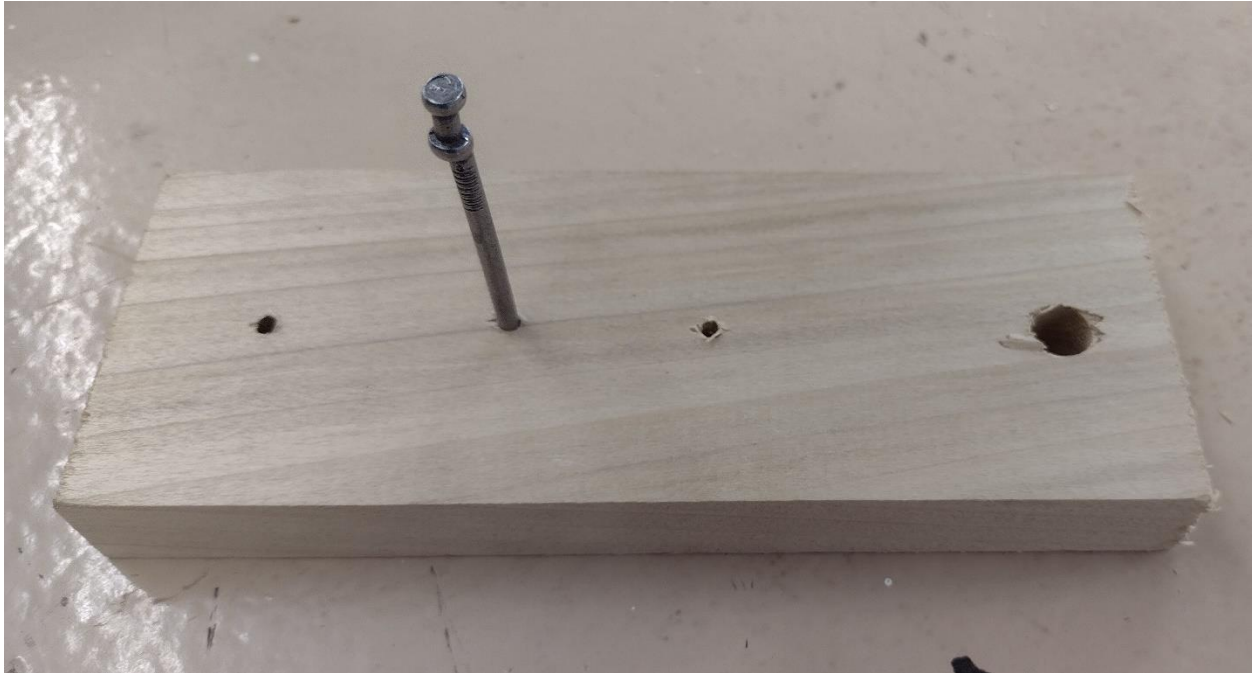
Holes drilled for nail.
