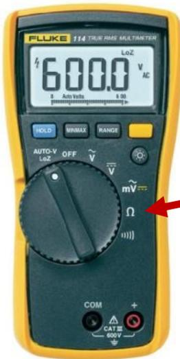
If you look at your tester when the probes are not touching anything, you should see a reading of infinity or OL. Touch the two probe tips together and you should see the reading change to zero. If your tester features an audio alert, it too will sound as you touch the probes together.
