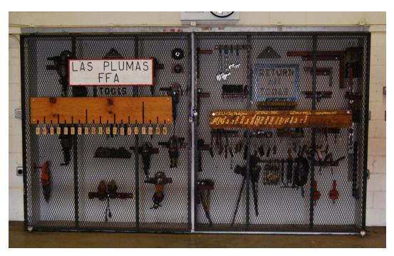
This type of tool storage is desirable since you can see what is stored even when locked.
