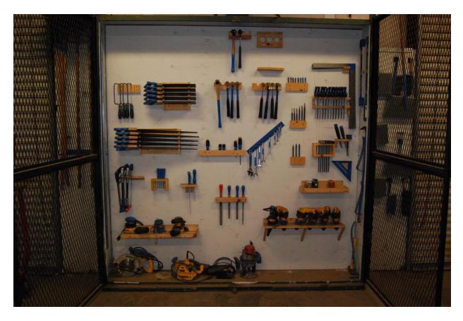
Cabinet with wood brackets and expanded steel doors.
