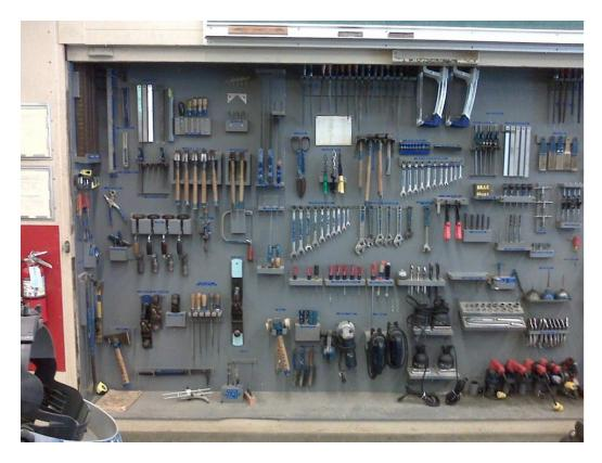
A good example of general tool storage with a vertical door. The vertical door does not take space.
