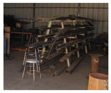
Steel is heavy and must be stored on sturdy racks. The "A" frame design is a common one that is easily constructed. Ideally steel storage is located under cover and easily accessible for loading (from a delivery truck) and the construction area.
