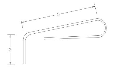
1/8"x3/4" HR drilled to match sheet metal and bent in bender. Size approximate.
