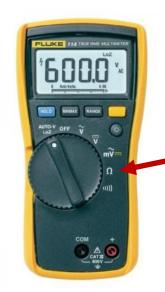
If you look at your tester when the probes are not touching anything, you should see a reading of infinity or OL. Touch the two probe tips together and you should see the reading change to zero. If your tester features an audio alert, it too will sound as you touch the probes together.
