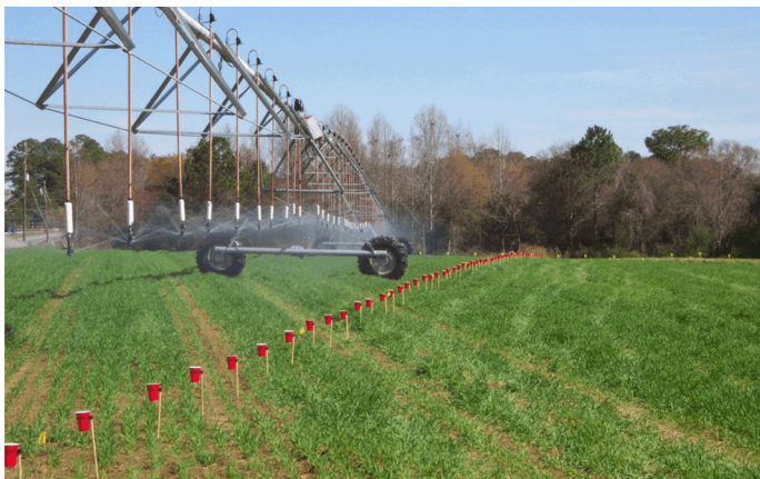
Figure 1. Catch cup layout using 16-oz drink cups as collection devices.
